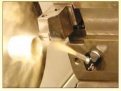
**TurretJets** are ideal for CNC Turning Centers, Machining Centers, Screw Machines and CNC Multi-Axis Grinders.
